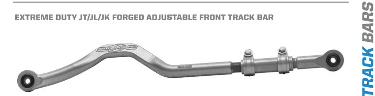
The Rubicon Express JK, JL & JT Wranglers front forged track bar features a heat treated steel construction designed to eliminate deflection caused by oversized tires or extreme side load. It features an adjustable sleeved collar which allows for precise axle alignment while still on the vehicle preventing the need to disassemble the suspension as well as OE style bushings.
