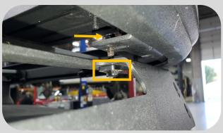
Insert the M6 bolt plate from the bottom to the top. Insert the M6 washers and nylock nuts and tighten using a 10mm wrench.
