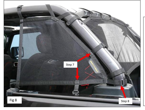
Step 8: Install the last strap as low on the roll bar as possible. Then even tighten all straps for a tight and even fit. Fig 8.
