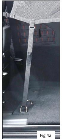
**Step 4:** Attach the bottom straps thru the footman loops on the floor of the jeep then back up to mesh and secure by running it through top loop and secure with Velcro. Fig 4a and 4b.
