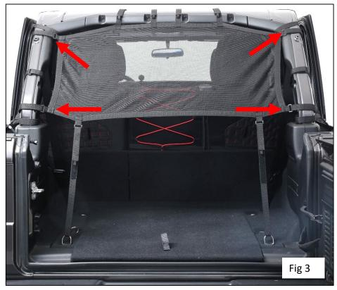
**Step 3:** Attach the remaining side roll bar straps ensuring mesh is centered. Then retighten the upper side roll bar straps. Fig 3
