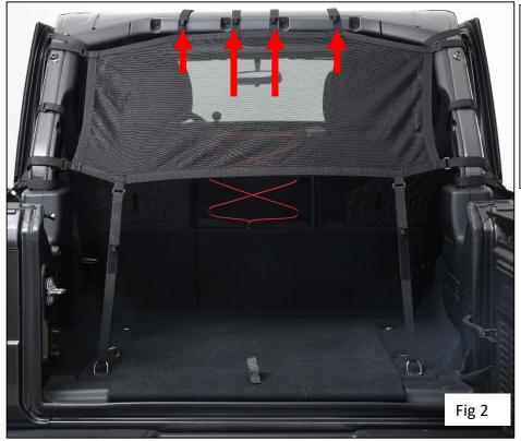
Step 2: Attach the top roll bar straps ensuring mesh is centered. This is easily accomplished by placing the two center most straps on the edge of the dome light. Fig 2
