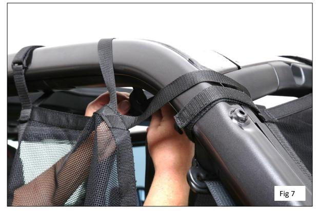
Step 6: Attach corner strap by putting each strap over the roll bar and securing them on the inside corner of the roll bar. Do not fully tighten. Fig 7.
