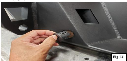
NOTE: For vehicles without back-up sensors, install block off plugs provided with the bumper, into the JT Gen 2 bumper instead.
