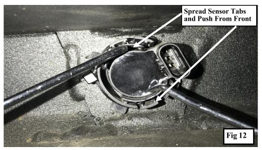
NOTE: Be sure to note the orientation of the back-up sensor retainers in the OE bumper prior to removal for reinstallation.
