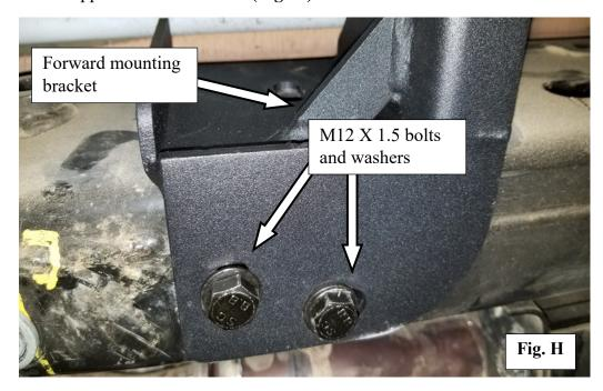
Step 11: Locate wired nut-plate. Bend the wire 90° at the nut-plate and insert it through the smaller hole in the frame (Fig. I). Run it up the frame and behind the for wardmost mounting bracket. Make sure that it is perpendicular to the frame with smooth side facing the mounting bracket. Secure with provided M12 X 1.5 bolt and washer, tighten hand tight. Repeat process on opposite side of vehicle.
