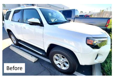
Note: due to vehicle variances, nerf bar to front mud flap clearance may vary. Mud flap may need to be adjusted to provide added clearance. This can be done by loosening mounting bolts and pushing forward on flap and then tightening bolts while pushing forward. Some cases may need to add a flat washer as a shim to space mud flap forward. This would need to be done on the bottom two mounting bolts.
