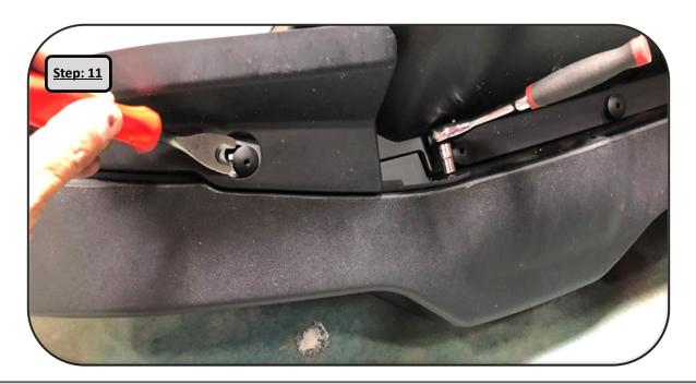
**Step 11:** Remove the OE plastic push rivets and any remaining screws. Remove the OE back panels from the OE front bumper.
