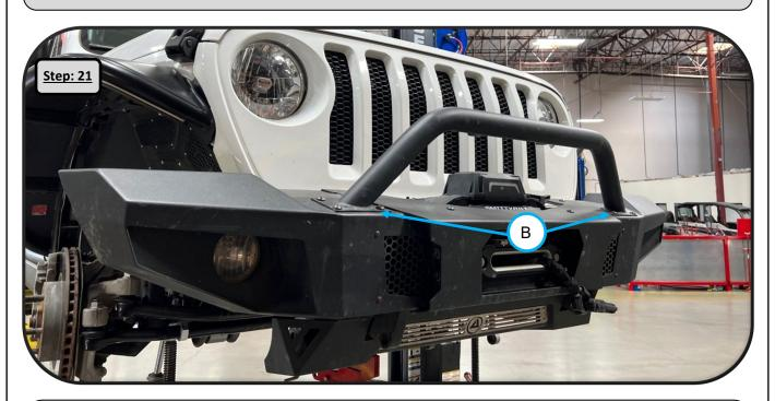
**Step 21:** With the help of a friend, mount the **Bumper Assembly** onto the **Winch Cradle**, and through the outer frame horn mounting holes. Secure using supplied M10 Washers and Locknuts, do not tighten this hardware yet.
