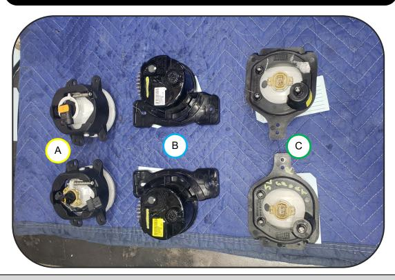
**NOTE:** Depending on trim level, there are three different styles of OE fog/driving lights. This kit includes adapter brackets for styles **A** and **B**, style **C** is direct bolt in.
