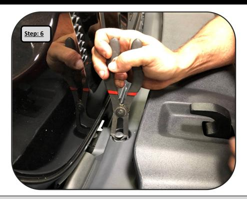
**Step 6:** Some models have optional beauty trim between the bumper and grille, go ahead and remove this by removing the plastic rivets securing it to the top of the frame rail. It will not be re-used
