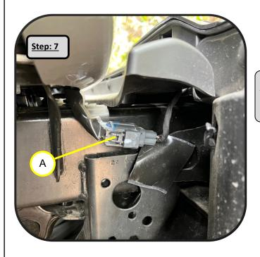
**Step 7:** On the Passenger side frame, behind the bumper, locate and disconnect the Bumper Harness Connector **(Fig A.)**
