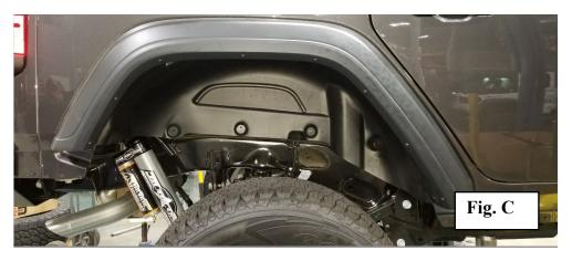
**NOTE:** You will hear cracking/ popping noises, this is normal, it's from the clips snapping (they will not be reused).
