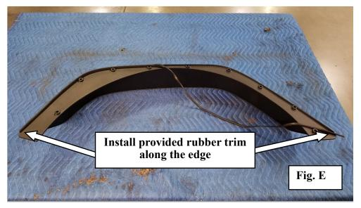
**Step 6:** With the help of a friend install the **Apollo Fender Flare**, start by lining up the fender with the O.E body panel holes, loosely install (2) of the provided M6 bolts into your previously installed nutsert. Loosely install the remaining hardware to the fender.
