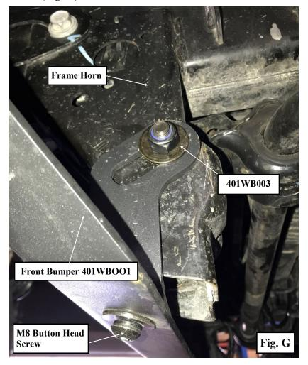
Step 10: Secure the (2 Per Side) front bumper lower mounting holes to the lower mounting tabs (84-401JB008 drvr and 84-401JB009 pass) using the supplied 8mm X 30mm bolts, washers, (Fig G)
