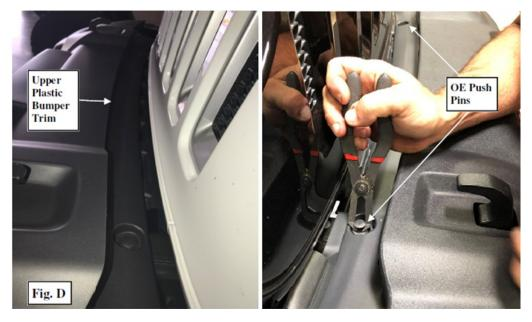
**Step 5**: Carefully remove the **OE front bumper** from the vehicle.
