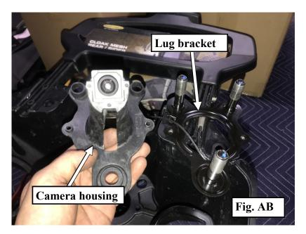
Step 28: Locate the Adjustable Wheel Mount Bracket (401TU034) and carefully install the OE camera housing and lug plate. Use the two (2) M6(1.0) X 20mm countersunk screws provided to tighten the assembly (Fig. AC). Set aside for now.
