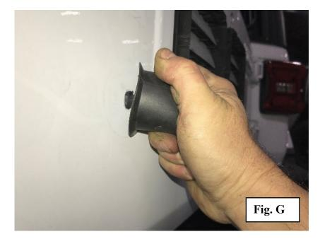
**<u>Step 6</u>**: Insert the two (2) push in plugs **Hardware Pack (60714)** into the two anti-rattle holes **(Fig. H).** The plug will snap into place with the outer edge flush to the door when properly installed.
