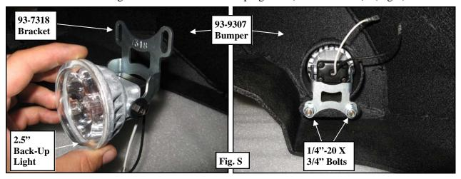
Step 20: Install the back-up lights into the new M1 rear bumper (93-9307) using the supplied (2 per side) 1/4"-20 X 3/4" bolt and hardware. (Fig S)
