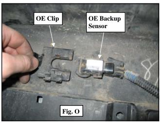
**Step 17:** Remove the **(2) OE** back-up sensor retainers from the **OE** bumper, if so equipped. (Fig P)
