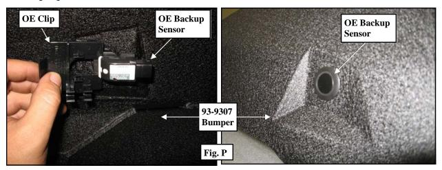
Step 18: Install the (2) back-up sensors into the mounting holes on the M1 rear bumper (93-9307) according to their original orientation in the OE bumper. Secure using the removed OE clips. (Fig R)
