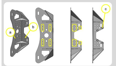
The Hi-Lift Mount can be mounted to the swing gate using face (a) or (b) as needed. After selecting which configuration to choose, one bolt must be secured in each of the 4 rectangles to ensure secure installation (shown at c).
