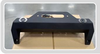
**Step 8: Install OE parking sensors into new location**
