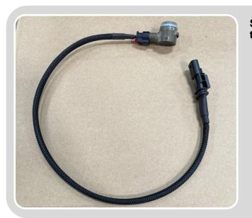
Step 7: Plug in sensors to wire harness extension 2X.
