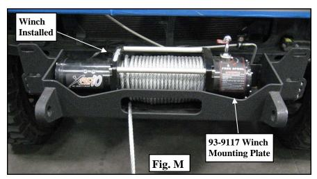
NOTE: Do not install the winch control box at this time. It will be installed later.
