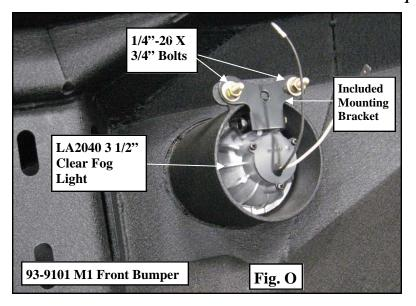
Step 21: Install the fog lights into the new M1 front bumper (93-9101) using the supplied (2 per side) 1/4"-20 X 3/4" bolt and hardware. (Fig O)
