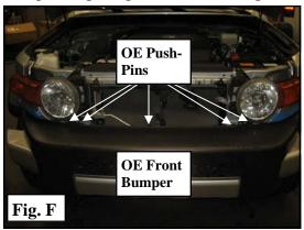
**Step 9:** Unclip the **OE** front bumper and carefully remove the bumper from the vehicle. Save  $\overline{OE}$  hardware for reinstallation. (Fig G)
