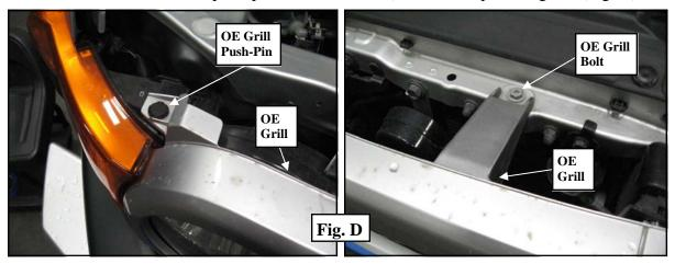
**Step 7:** Carefully release the **OE** plastic retainers and remove the grill. (Fig. E)
