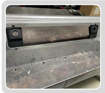
Steps 14-17 are for parking sensor wire harness installation to bumper. If not installing harness proceed to Step 18. Use PN: 90-60840 panel plugs to cover sensor holes in bumper.
