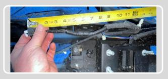
Note: If installing sensors without winch cradle, apply & adjust wire harness as shown in Step 16. If using winch cradle, use wire hardness extension from winch cradle instructions.
