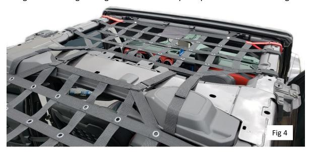
**Step 6.** Rear main netting should be attached securely around sound bar. Then loosely attach all side straps while your working your way back and over the rear roll bar. Front most side strap should be as close to the sound bar as possible. Tighten both front side straps evenly and work your way towards the back pulling the netting tight as you go back. Fig 5.
