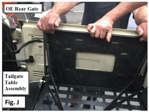
**Step 3:** Remove the tailgate table assembly and center punch the previously marked holes to prepare for drilling.
