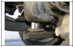
Install the 1" spacers between the differential supports and the front cross-member. Install the new bolts with factory washers and the new nuts and washers. Torque to factory specs.
