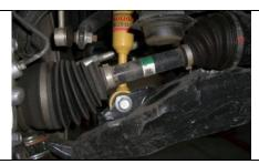
2. Starting from the passenger side, loosen the up-per and lower strut mount nuts.
