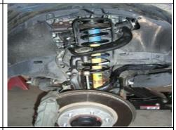
6. Reinstall the strut assembly in its stock location. Leave the three upper strut mounting nuts loose Raise the lower control arm and install the lower strut mounting bolt and nut. Use a floor jack to raise the lower control arm up in order to get the lower ball joint bolts installed. Be sure to use a thread locker on the lower ball joint bolts. Be sure to tighten all nut and bolts to factory specs.
