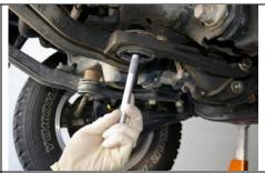
Remove the factory 19mm differential mounting nuts and bolts. The OEM washers will be reused.
