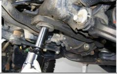
Position a floor jack under the front differential. Raise the pad so that it is touching the diff.
