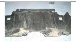
**1**. Remove the skid plate by unbolting the four 12mm bolts.
