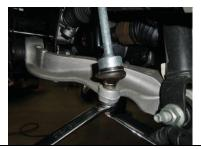
5. Carefully strike spindle to break upper ball joint loose.
