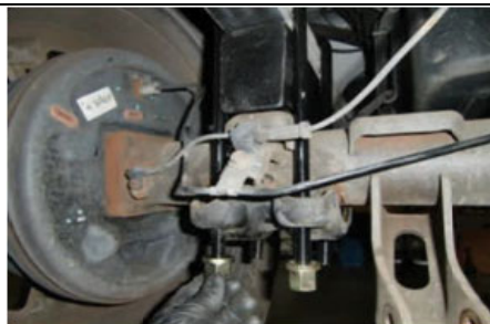
Install new, longer, U-bolts and hardware.
