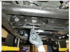
Now, install torsion key adjuster bolt and adjust for initial setting. Final adjustments will be done during alignment.
