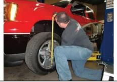
Measure ride height then lift vehicle and remove wheels/tires.
