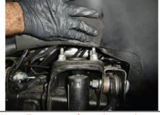
Note: To prevent damaging torsion bar tool. Peel back wheel well liner and remove (2) upper shock mounting nuts.
