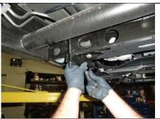
With torsion bar tool remove adjuster bolt.
