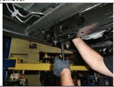
Use torsion bar loading tool and adjust new forged torsion key up just enough to allow adjuster block to be reinstalled.
