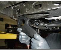
Install new forged torsion keys into position and slide torsion bar into hex as original.
