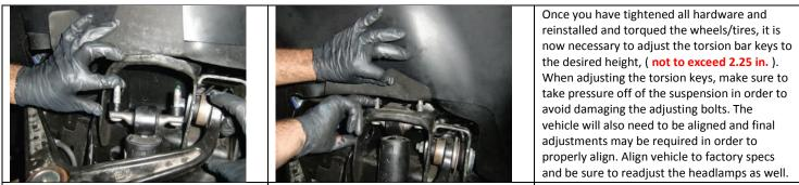
Picture shows spacers being installed onto upper studs.
