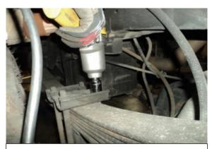
Remove U-bolt nuts on top of spring pack.
