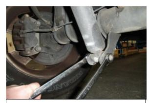
Remove the lower shock mount hardware.
