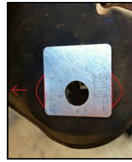
0 degree change from stock. Use like this to weld onto bracket as a repair to a worn out hole
